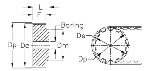
Type = AT10Belt width = - 16 mm Weight = 1.09= 150.95De Dm = 95 = 76.4Dp F = 21 L = 31 Pre-drilled = 16
